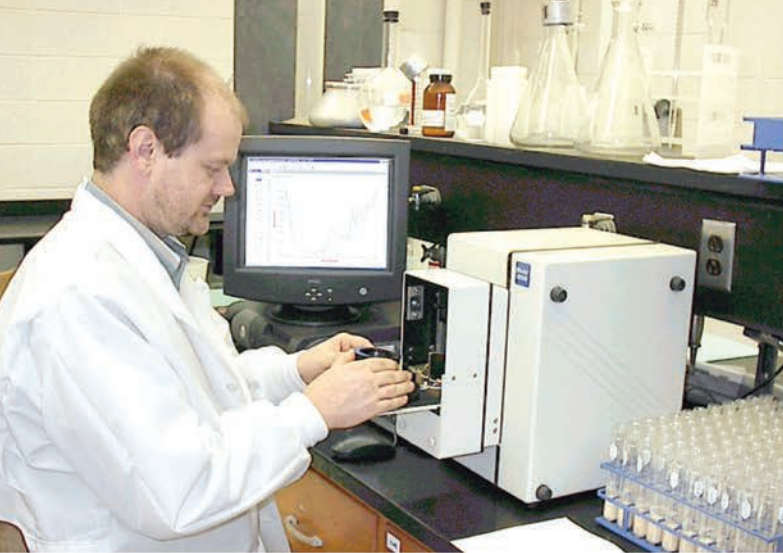
Left: A researcher prepares samples contained in scanning cups to be scanned in a benchtop near-infrared spectrometer. Right: Grass sample ready to be scanned using a handheld spectrometer. Photo on the right courtesy of Miguel Castillo.
